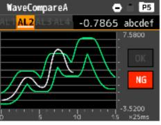
It is possible to judge not only the pressure level but also the concept of time. High-speed sampling of 4000 times / sec at the fastest
